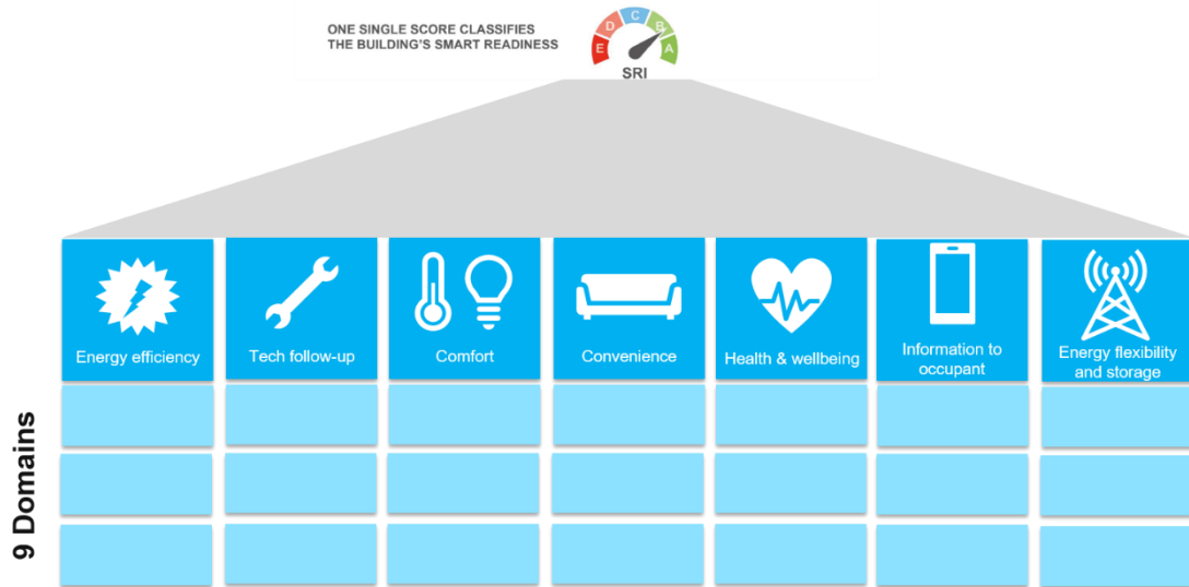
Figure 18 - Seven impact criteria as suggested by the first technical study on the SRI
