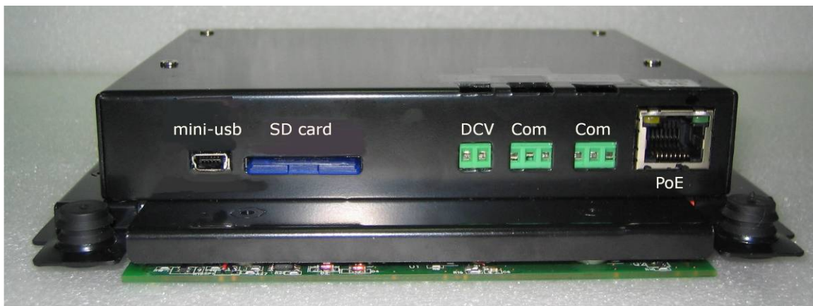
CE 5.0 embedded OS + RS232 (3-wire) Ports + PoE
