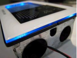
CE 5.0 embedded OS --- RS232 (3-wire) Ports --- Blue LED edge light pipe
