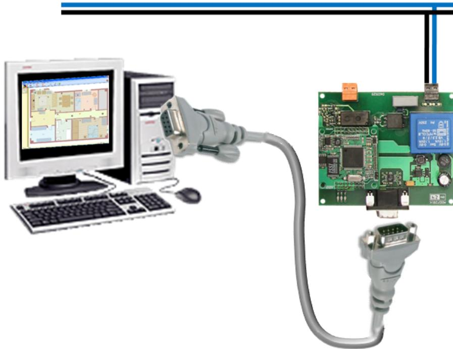
Next, power the board up and launch C@sa application. ADD7281 serial communication baud rate is 57600. Then, PLC network can be controlled and monitored.
